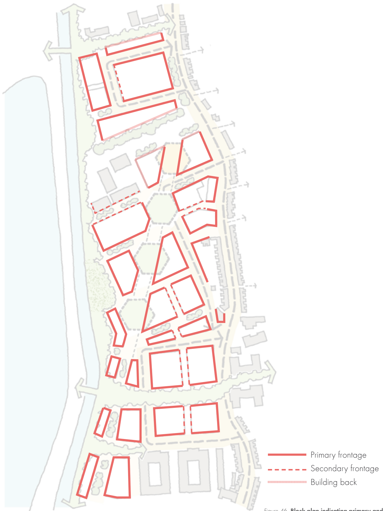
Figure 46 Block plan indicating primary and secondary frontages as well as building backs
