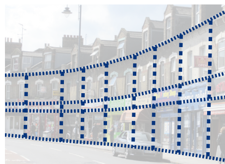
A cohesive approach can be achieved along the street by following vertical lines set out by pilasters, and horizontal lines established by cornices and fascia
