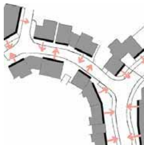
A varied building line can create oblique views across the street. Image taken from 'Better Places to Live'.
